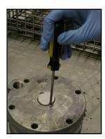
To remove the heating element it is best to remove the puraDYN system from it mounting location to access the bottom of the PFT Unit where the heating element is located.
