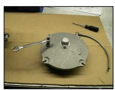
Using a wrench or socket (size 9/16), unscrew the vent valve from the TF Lid (left) or PFT base (right).
