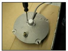
The heating element is located top dead center of the Lid.
