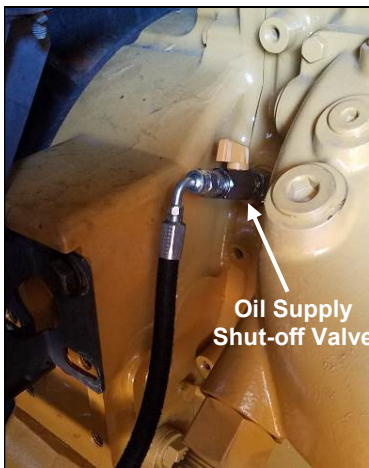
Picture 4 (Oil supply Shut-valve- C32)
