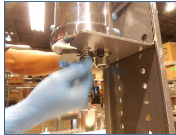
3) Rotate fitting CCW, to remove- metering jet screen will drop down- if screen does not drop, use probe tool to gently dislodge
