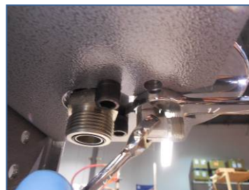
7) Slightly unscrew fitting- as required to orient fitting facing forward (or in direction required for install), then use (2) wrenches to hold fitting in place while tightening locknut
