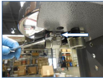
2) Loosen (adjustment) locknut on 90 Degree fitting- allowing rotation of fitting
