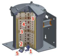
STEP 1. OIL ENTERS SYSTEM AT SLOW RATE OF 6-8 GPH / 22-40 LPH AND INTO THE INNER DISPOSABLE ELEMENT WHERE THE FOLLOWING PROCESSES OCCUR:
