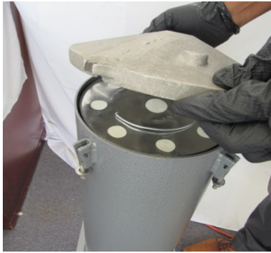
1. Line up torque bolts with slots on lid, and place lid centered on top of canister rim to get a proper seal.
