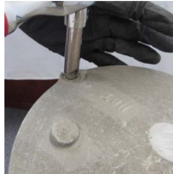
5. On corresponding number 2 , tighten lid bolt with 8 no. of ¼ (90-degree) wrench turns ( do not exceed 8 no. of ¼ wrench turns )
