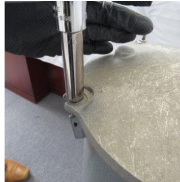
6. On corresponding numbers 3 and 4 , tighten lid bolt with 6-7 no. of ¼ (90-degree) wrench turns ( do not exceed 8 no. of ¼ wrench turns )
