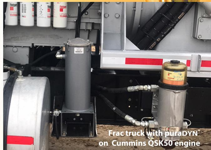
Frac truck with puradYN on Cummins QSK50 engine
