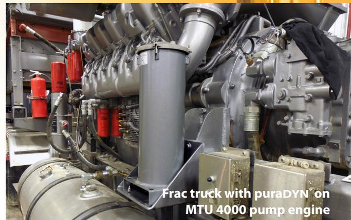
Frac truck with puradYN on MTU 4000 pump engine
