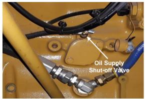
Picture 5 (Oil supply Shut-valve - C32)
