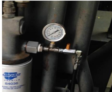
**Picture 6 (Oil supply Shut-valve - MTU16V2000)**
