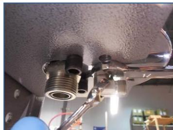
7) Slightly unscrew fitting- as required to orient fitting facing forward (or in direction required for install), then use (2) wrenches to hold fitting in place while tightening locknut
