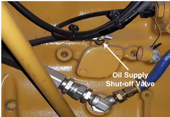
**Picture 5 (Oil supply Shut-valve - C32)**
