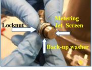
6) Place screen on face of fitting, centered, against dabbed oil; screw <u>this end</u> of fitting into port- by hand, until back-up washer contacts face of port.
