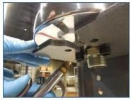
4) Clean port internals & metering jet screen with solvent/fine wire brush; use high-pressure air to blow-out port & screen, clearing any debris
