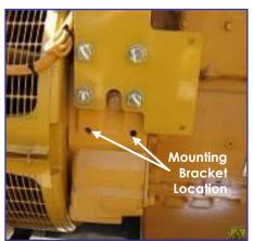
**Picture 3 - Mounting Locations** *Actual equipment application not shown*
