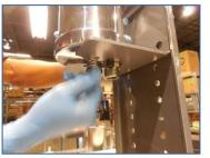
3) Rotate fitting CCW, to removemetering jet screen will drop down- if screen does not drop, use probe tool to gently dislodge
