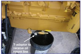
**Picture 9 - Oil Return Kit** Actual equipment and hardware not shown
