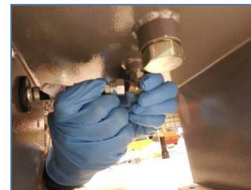
7) Slightly unscrew fitting- as required to align with hose assembly, then use (2) wrenches to hold fitting in place while tightening locknut; reconnect hose assembly
