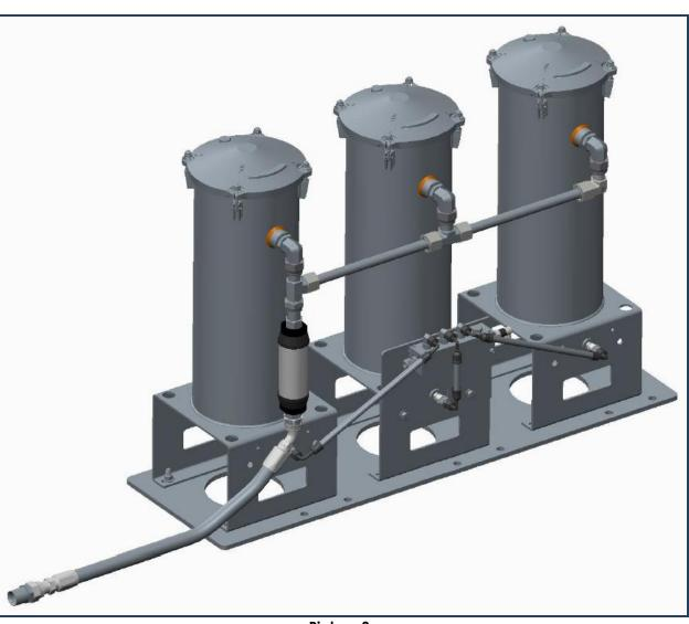
Picture 8 (Return Plumbing, Flow Meter and Return Hose set-up)
