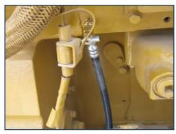
For Pressure Manifold Assembly connections, note that (1) end of assembly features a Push-Button Sample Valve, while the other end features a compression fitting for connection to supply
