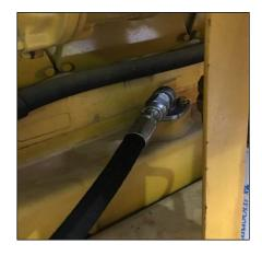
**Picture 7:** Return Fitting Assembly & Return hose connection
