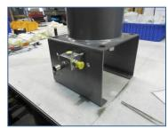
8) Check all fittings for tightness, then re-tighten locknut- securing FPS Manifold Assembly to unit base
