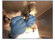
7) Slightly unscrew fitting- as required to align with hose assembly, then use (2) wrenches to hold fitting in place while tightening locknut; reconnect hose assembly
