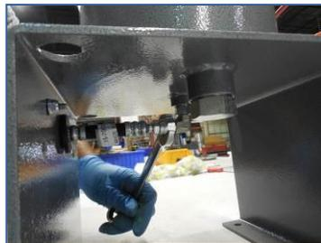
2) Loosen hose fitting, to disconnect 'Inlet Plumbing Hose Assembly'
