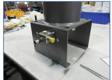
8) Check all fittings for tightness, then re-tighten locknut- securing FPS Manifold Assembly to unit base
