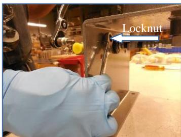
1) Loosen locknut, which secures FPS Manifold Assembly to unit base
