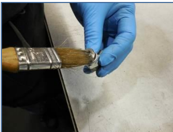
5) Back-off locknut/back-up washer on 90 degree fitting and lubricate external o-ring w/system fluid, also applying a dab on face of fitting- for screen adherence
