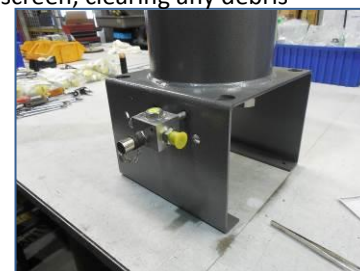
8) Check all fittings for tightness, then re-tighten locknut- securing FPS Manifold Assembly to unit base
