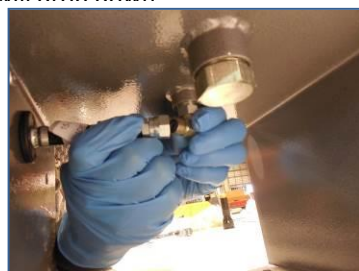
3) Loosen (adjustment) locknut rotate entire fitting CCW to remove- metering jet screen will drop down
