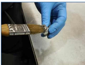
5) Back-off locknut/back-up washer on 90 degree fitting and lubricate external o-ring w/system fluid, also applying a dab on face of fitting- for screen adherence
