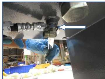
3) Loosen (adjustment) locknut rotate entire fitting CCW to remove- metering jet screen will drop down
