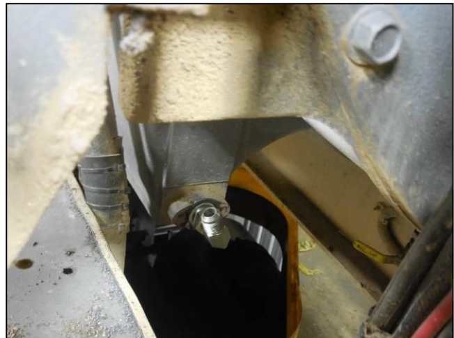
Picture 14: Lower, Rear of Oil Sump-Return Fitting Location
