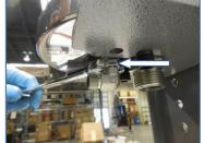
2) Loosen (adjustment) locknut on 90 Degree fitting- allowing rotation of fitting
