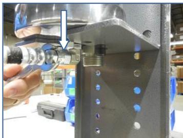
1) Loosen hose fitting, for disconnection of Supply Hose Assembly
