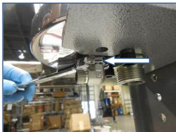
2) Loosen (adjustment) locknut on 90 Degree fitting- allowing rotation of fitting
