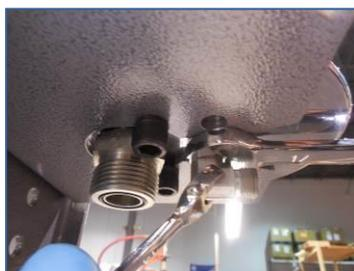
7) Slightly unscrew fitting- as required to orient fitting facing forward (or in direction required for install), then use (2) wrenches to hold fitting in
