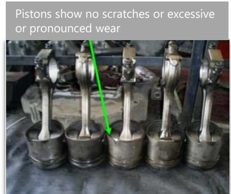
Pistons show no scratches or excessive or pronounced wear
