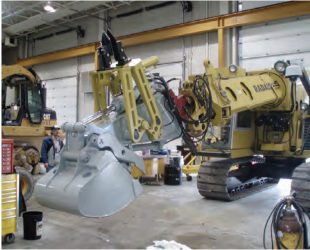
The bucket on the excavators was also specialized to incorporate a knuckle boom, narrow ditching bucket with a thumb and splaying tool.
